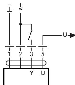
Override control and limiting with AC 24 V with rotary switch
