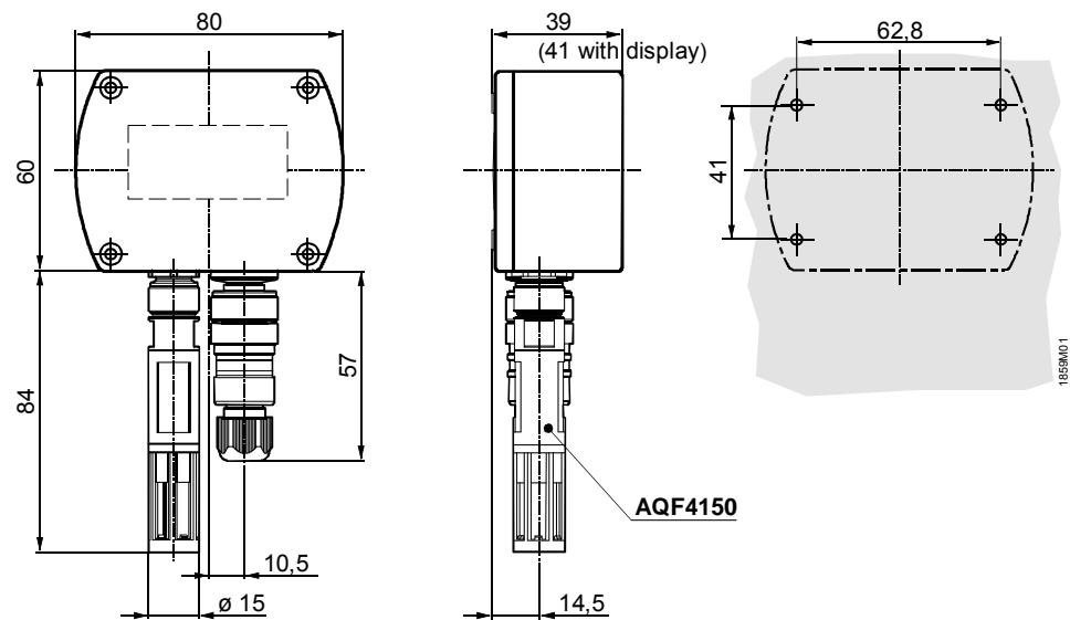
Dimensioning without (with) LCD-display
