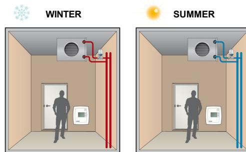
In 4-pipe installations, there are two separate pipe systems for heating and cooling with separate valves. The thermostat uses two outputs for control of heating and cooling in sequence.
